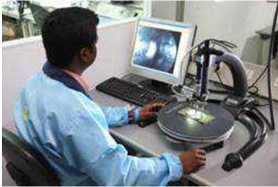
BGA underscope inspection
