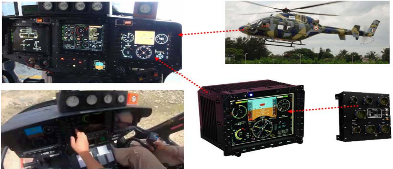
Light Utility Helicopter Cockpit display
