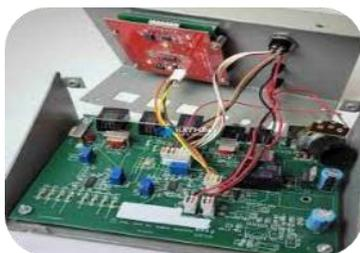
Also known as systems integration, box builds can be anything from a simple PCBA housed in a small enclosure, to a cabinet housing a complex electromechanical system. The box build process involves enclosure fabrication, assembling the various PCBAs and cables harness assemblies, installation of sub-assemblies and components and routing of cabling or wire harnesses.
