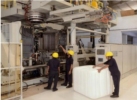
*Manufacturing of rigid Intermediate Bulk Containers*
