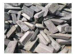
**9. Sponge Iron-** It is the product of reducing iron oxide in the form of iron ore and steel plant wastes into metallic iron, below the melting point of iron and typically in the range of 800–1200 °C. Sponge iron is used in the iron and steel industry as a substitute for scrap in induction and electrical arc furnaces. Over the years, the shortage of expensive melting scrap has made sponge iron a significant raw material for manufacturing high quality steel.
