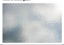
This technique uses hydrofluoric acid to achieve the frosted look of the glass. The acid reacts with the glass, corroding its surface and therefore providing it with its milky appearance. After the process of acid-etching, the glass experts thoroughly wash the glass, leaving behind permanently etched glass.
