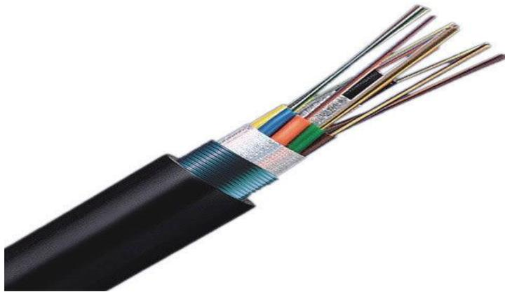
This cable is designed in such a way to withstand the mechanical stresses applied to overhead lines due to environmental factors such as wind and ice. It must also be capable of handling electrical faults on the transmission line by providing a path to ground without damaging the sensitive optical fibers inside the cable.
