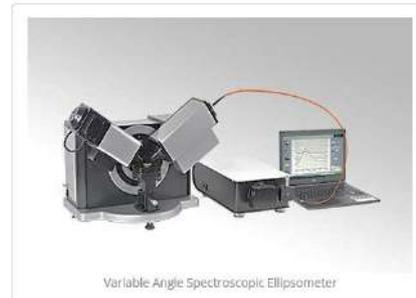
Variable Angle Spectroscopic Ellipsometer
