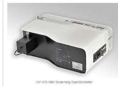
UV-VIS-NIR Scanning Spectrometer
