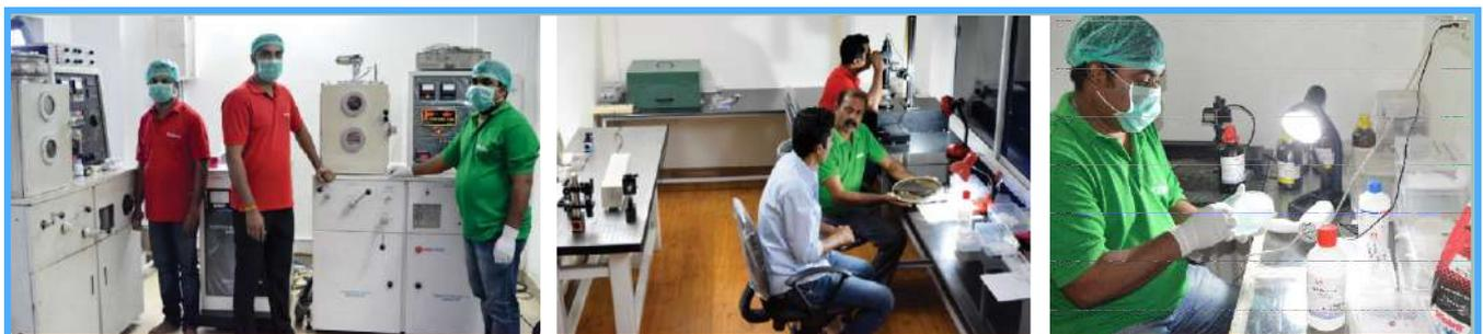
The Thin Film Coating Lab at Holmarc uses Vacuum coating chambers, Thin film reflectometer, Spectroscopic ellipsometer and spectrophotometers that aid in the creation of thin film optical coatings. A team of experienced engineers and technicians design, deposit, and measure thin film coatings ranging from our standard anti-reflective coatings to metallic mirror coatings.
