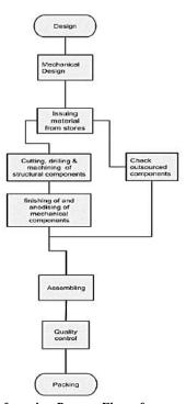
Manufacturing Process Flow of: Solid breadboard, Kinematic mirror mounts, Gimbal mirror mounts, Lens mount, Linear translation stages, Vertical translation stages, Goniometer, Rotation stages, Linear slide
