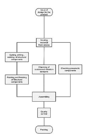
Manufacturing Process Flow of: Passive vibration isolation support
