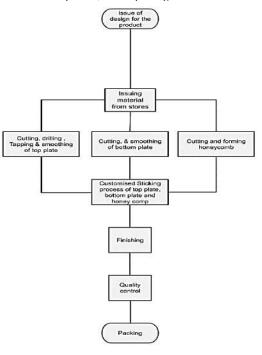
Manufacturing Process Flow of: Optical Breadboard
