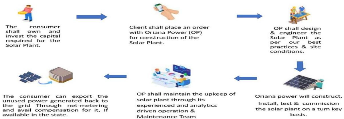
EPC refers to companies that deal with the Engineering, Procurement, Construction and Commissioning of solar systems. The EPC service provider is responsible for delivering a complete Photovoltaic (PV) power plant to the Asset Owner, handling all aspects from seeking authorisation for the construction to commissioning and securing a grid connection.
