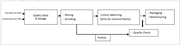
*Inspection of Raw Materials:* Upon delivery, the incoming materials are inspected pursuant to quality control specifications. Raw materials are accepted only after they have passed the relevant quality control tests.
