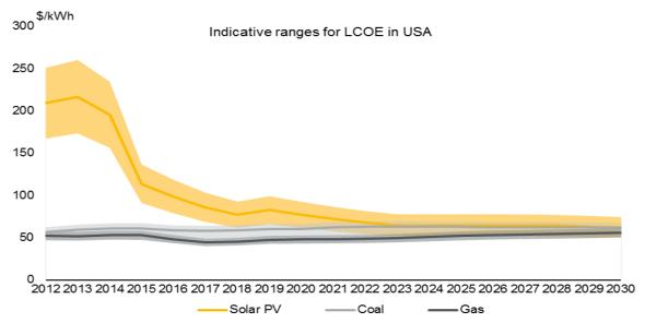
$Notes: Real\ 2017\ USD,\ Coal\ -\ scrubbed\ super\ critical,\ Gas\ -\ combined\ cycle\ steam\ turbine\ (CCGT)$
